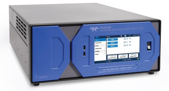
The Model T200P provides measurements of NO, NO<sub>x</sub> and NO<sub>2</sub> using our T200 analyzer combined with a patented high efficiency Blue Light Converter (BLC). The BLC, also known as photolytic converter, provides a very specific conversion of NO<sub>2</sub> with conversion efficiency similar to molybdenum.\*
