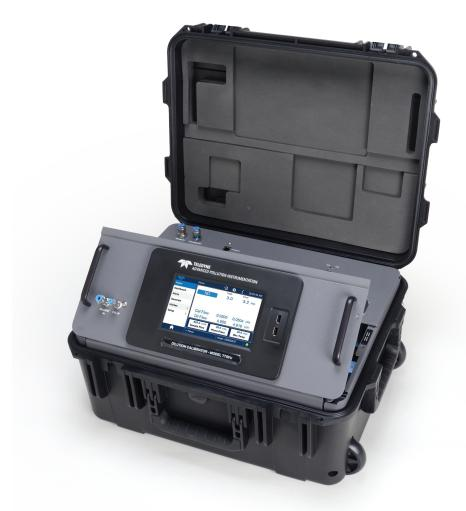
A portable, microprocessor based calibrator for precision gas analyzers, the Model T750 combines highly accurate mass flow controllers and compressed sources of standard gases to provide multipoint span and zero calibrations. The T750U includes two operating modes: a high range with similar performance to the Model T700 instrument with ozone generator, and a low range which includes a "fractional mode" for producing accurate and stable O<sub>3</sub> and NO<sub>2</sub> levels down to 3 ppb.
