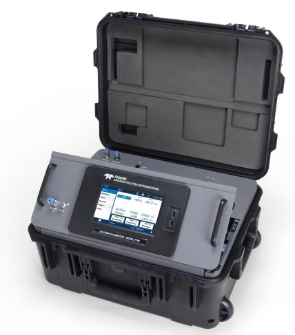
A portable, microprocessor based calibrator for precision gas analyzers, the Model T750 combines highly accurate mass flow controllers and compressed sources of standard gases to provide multipoint span and zero calibrations. UV ozone generator, photometer, and gas phase titration (GPT) chamber options are also available for the T750 for stable and accurate O<sub>3</sub> and NO<sub>2</sub> production.
