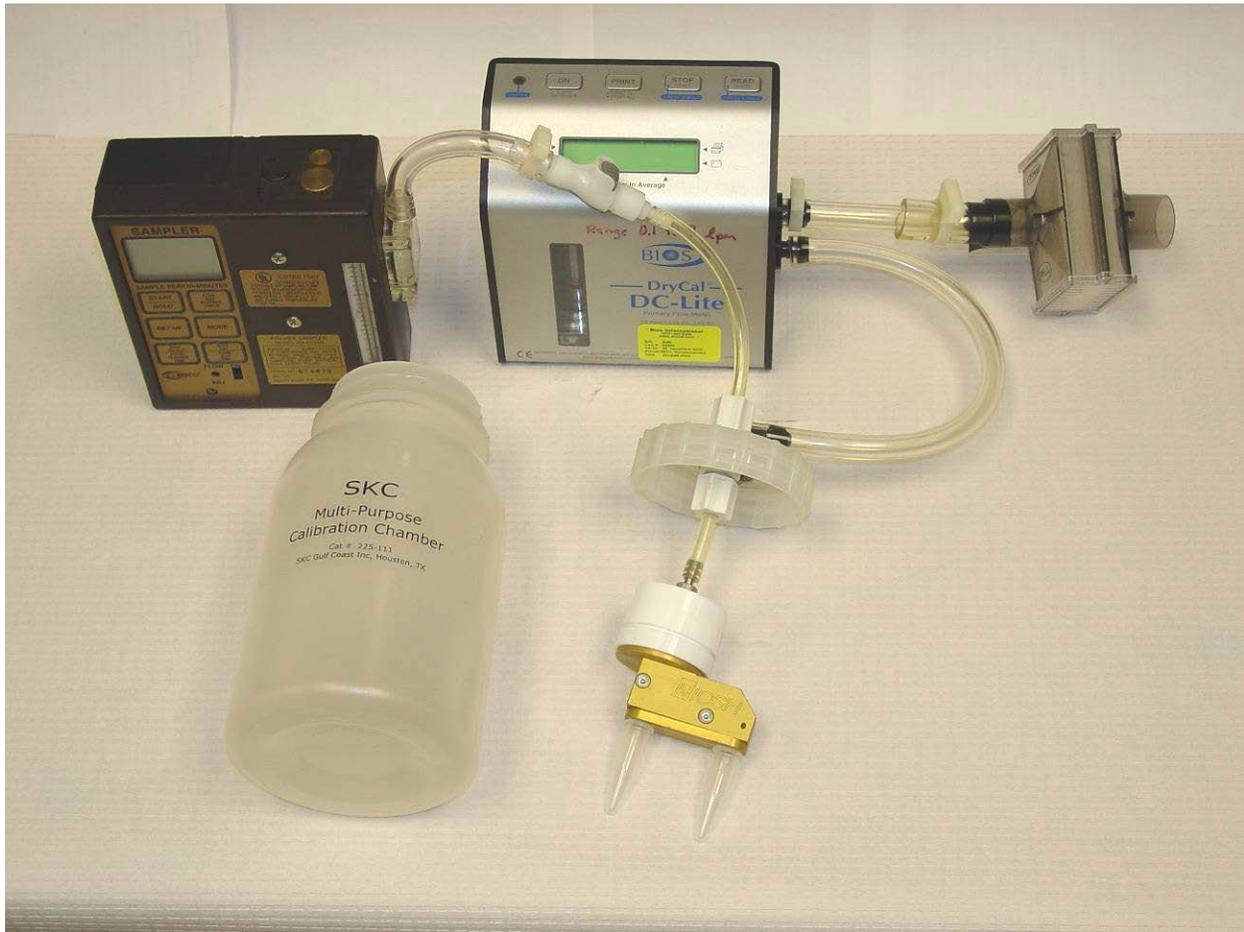
**Flow calibration.** The airflow through the sampler must be calibrated before each use. A calibration jar may be used for this purpose. SKC makes a large calibration jar (#225-112) that will fit all of the samplers, including the BC 251. Attach the sampler to the fitting as shown and place it in the jar. Connect the pump and flow meter. Turn the pump on and allow it to warm up for 5 minutes before setting the flow rate.
