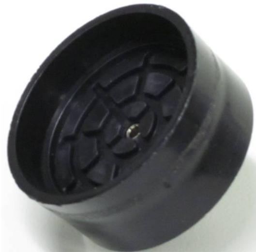
This metal Luer fitting in the center of the cassette fits properly. The tip of the fitting is at the bottom of the channels in the gridded surface, which allows air to flow through the channel and into the fitting.
