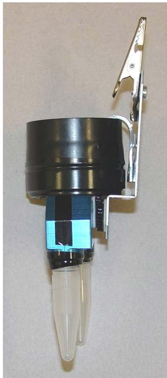
**Side view of BC 221:** Clothing clips are mounted on aluminum holders. The holders have black Dual Lock strips for fastening to the back of the sampler. A split round nylon retainer is also used to help hold the sampler more securely.
