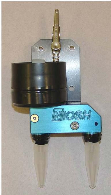
**BC 221 sampler:** The tubes and filter cassette on the BC 221 are sealed with tape as shown rather than caulk. The seam around the sampler is sealed with tape to prevent air leakage during use. The filter cassette is black conductive polypropylene.
