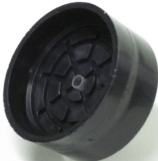
This plastic Luer fitting in the center of the cassette does not fit properly. The tip of the fitting is protruding above the top of the channels in the gridded surface. The filter support pad will press against the tip of the fitting, obstructing the flow.
