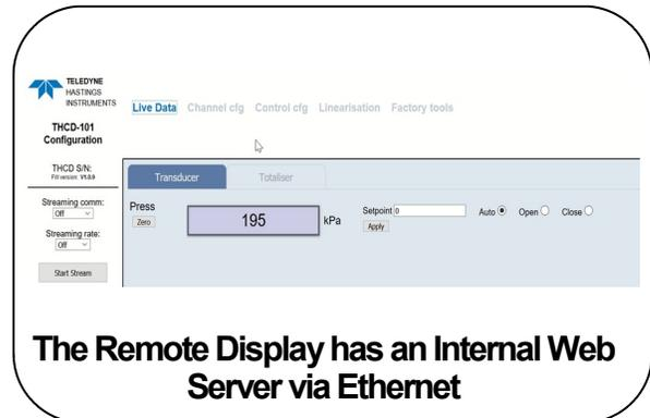
The Remote Display has an Internal Web Server via Ethernet
