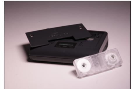
The microAeth® MA300 is a small, real-time 5-wavelength UV-IR Black Carbon monitor with an 85 sampling location automatic filter tape advance system which allows for 3-12 months of continuous measurements.
